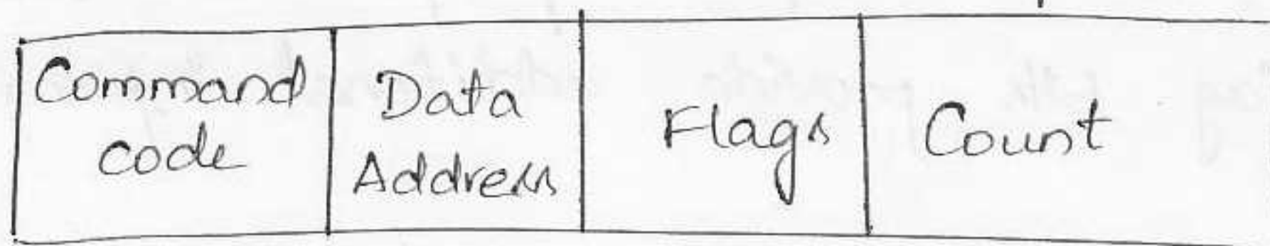
(c) Channel command word format
